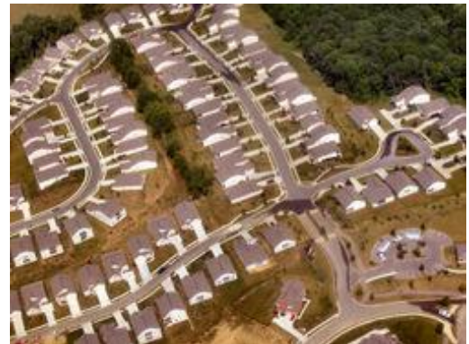
Curvilinear street patterns and few intersections in this conventional subdivision reduce the number of paths available to drivers and pedestrians.
